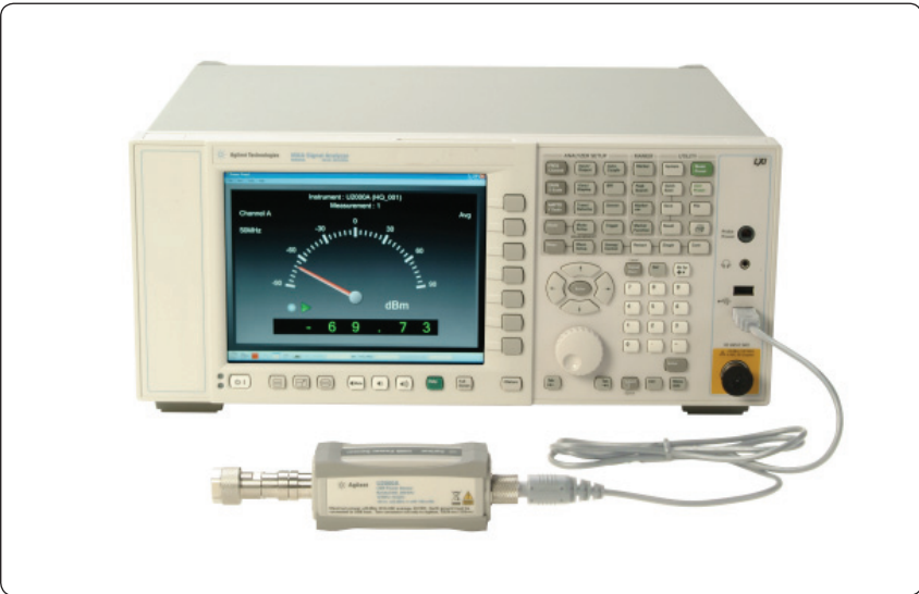
Figure 8 Intelligent instruments like the Agilent N9020A MXA Spectrum Analyzer can add accurate power measurements to their other capabilities by attaching a U2000 Series.
