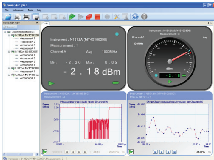
Figure 11 The Power Analyzer shows a powerful customizable display configuration of various data inputs. In this case, four completely different types of measurement processes are displayed in a single tab.
