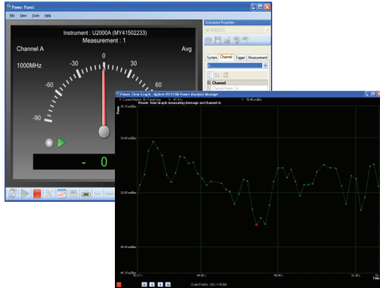
Figure 4 Strip chart continuous analog monitor of a power channel.
